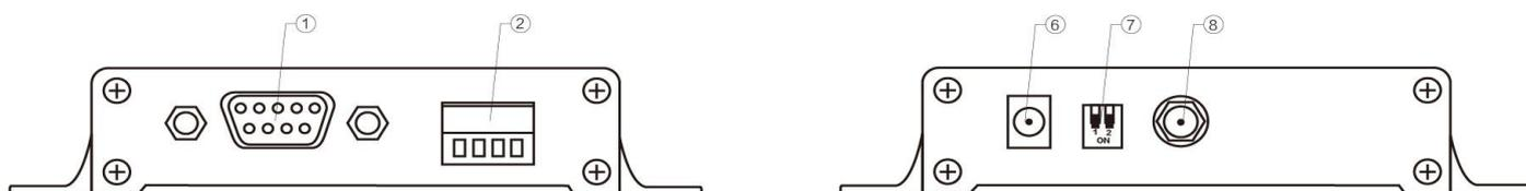
Users can choose ⑥ DC power interface, using the power adapter supply with the interface of the 5.5mm outer diameter, 2.5mm diameter;
