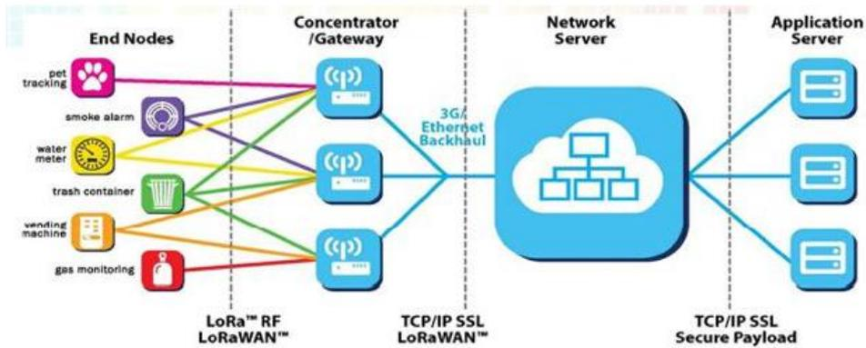
The complete LoRaWAN network system consists of nodes, gateways, LoRa Network Server, application servers, nodes typically designed by LORA chips, and gateways by Semtech SX1301 Design; LoRa Network Server now has open source loraserver or commercial TTN(The Things Network) that users can build on their own, and application servers are developed by user-defined designs and are primarily used for data exchange with LoRa Network Server applications.
