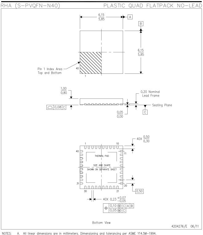
All linear dimensions are in millimeters. Dimensioning and tolerancing per ASME Y14.5M-1994. Α.
