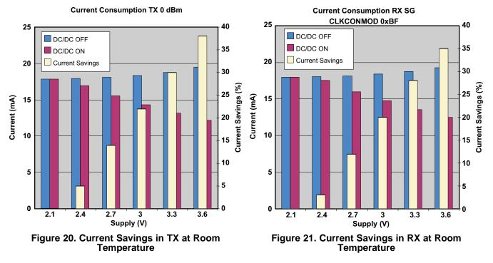
The application note (SWRA365) has information regarding the CC2541 and TPS62730 combo board and the current savings that can be achieved using the combo board.
