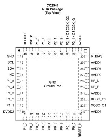
NOTE: The exposed ground pad must be connected to a solid ground plane, as this is the ground connection for the chip.
